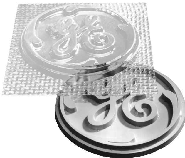
Fig.1.14: Typical Vacuum Forming Mould
